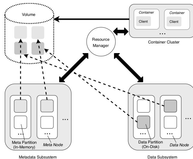
CFS consists of a *metadata subsystem*, a *data subsystem*, and a *resource manager*, and can be accessed by different *clients* (as a set of application processes) hosted on the containers through different file system instances called *volumes*.
