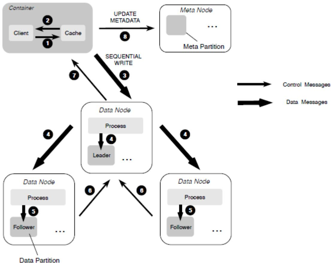
When overwriting an existing file portion during random writes, we employ a MultiRaft-based replication protocol, which is similar to the one used in the metadata subsystem, to ensure the strong consistency.
